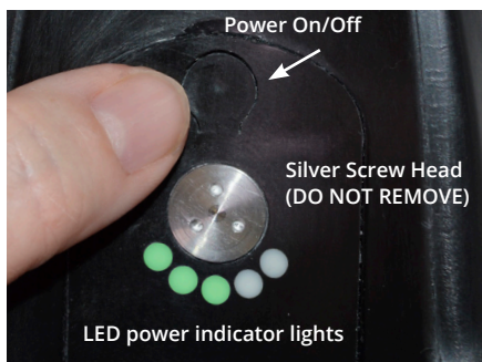
The power button and red/green LED indicator lights are located on the front of the elbow.
